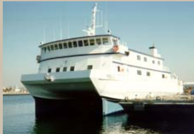
Western Flyer 117' x 53' SWATH Equipped with Two Aluminum HT 400's
